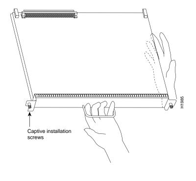
Note Leave the interface processor filler installed in any unfilled interface processor slots.
